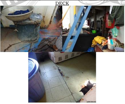
Pictures of other deficiency: OILY, UNNECESSARY ITEMS SCATTERED ENGINE ROOM
